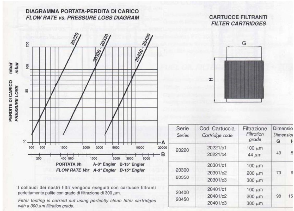
Filter testing is carried out using perfectly clean filter cartridges with a 300 µm filtration grade.
